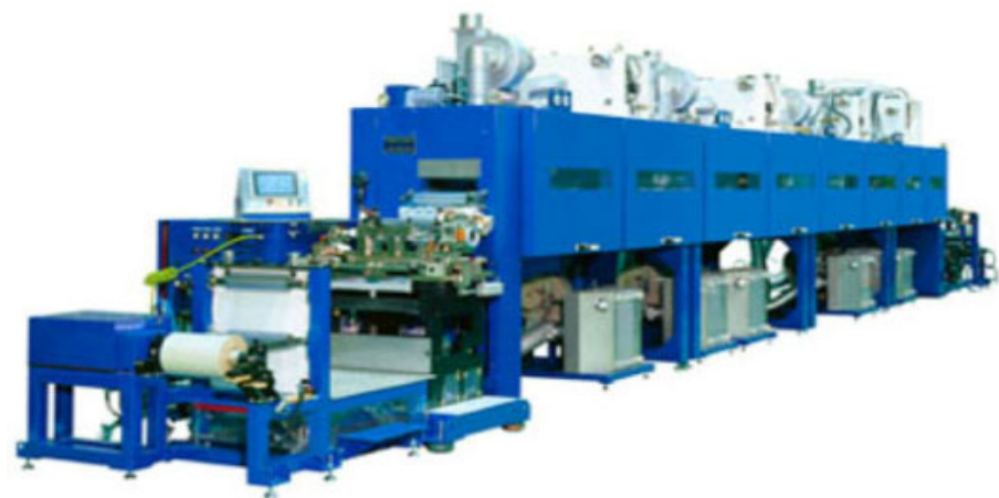
陶瓷电容涂布机 Coater for ceramic capacitor
