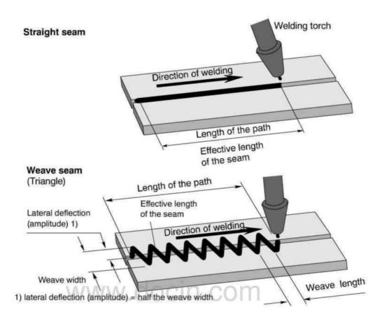
Trapezoidal, spiral and figure-of-eight weave patterns also result in a non-uniform effective weld velocity. This can vary between the set path velocity and a multiple of it during one period, depending on the relation of the lateral deflection (amplitude) to the weave length.
