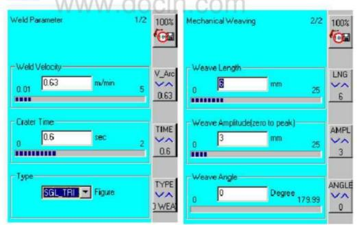
Enter the welding velocity (Weld Velocity) and the crater filling time (Crater Time).
