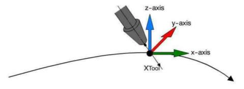
The tool-based moving frame or TTS (toolbased technological system)
