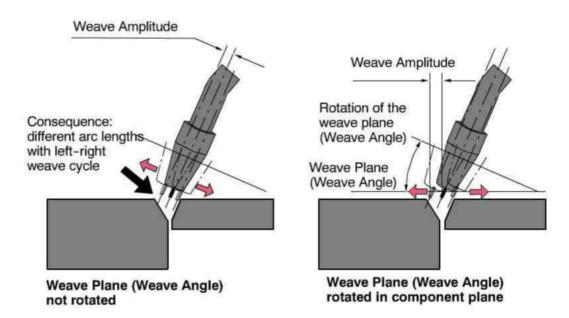
In certain applications, the welding result can be specifically influenced by rotating the weave plane. This requires appropriate tests to be carried out beforehand, however.
