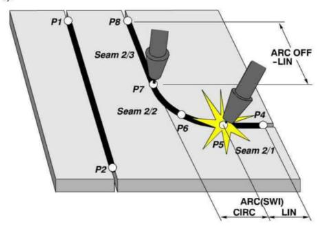
The first section of the seam is programmed as "ARC SWITCH" with the motion type "LIN" and the second section as "ARC SWITCH" with the motion type "CIRC". The command "ARC OFF" with the motion type "LIN" ends the seam.
