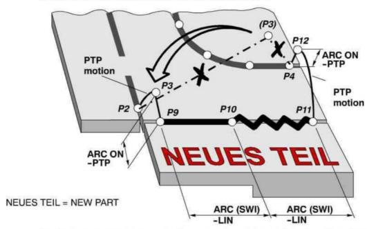
For design reasons, this seam for the new part must be welded using different parameters: it is to be welded as a normal straight seam in the first section and mechanical triangular weaving is to be used in the second.
