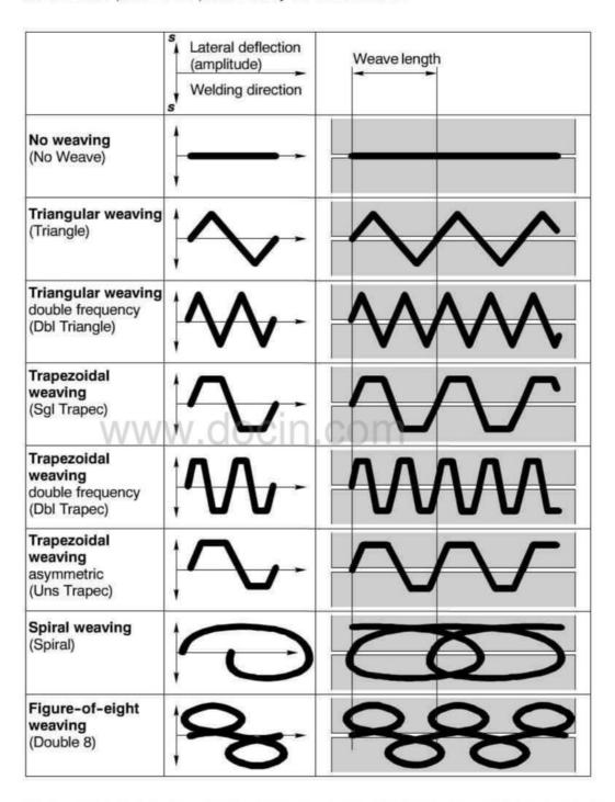
The lateral deflection (amplitude), the weave length (the length over which a pattern is executed) and the angle of the torch to the welding plane can be set for each weave pattern.
