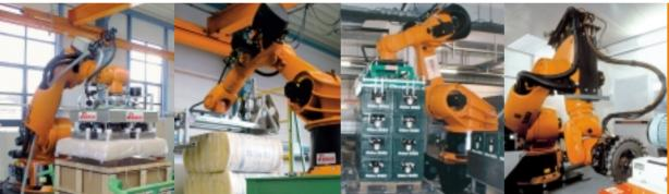
Through appropriate limitation of the heavy-duty robot's work envelope it was possible to increase the carrying capacity of the palletizing variant significantly. This special feature results from the downwards-pointing position of the robot wrist during palletizing.
