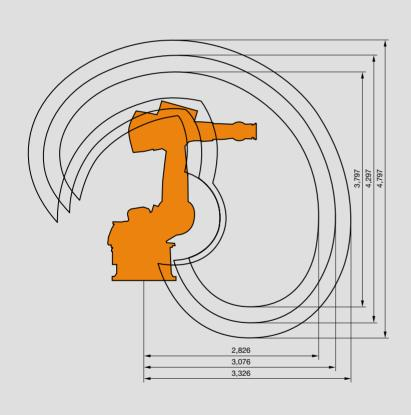
The fist-shaped work envelope of the standard KUKA heavy-duty robot can be made twice as large through the use of arm extensions. With its combination of long reach and high carrying capacity, the KR 500/1 is the KUKA heavyweight champion.
