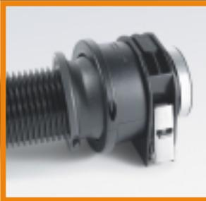
**Ball joint:** The cable and hose bundle ends in a ball joint at the robot wrist flange. This reduces the stress on the bundle during rotational motions of the wrist and ensures optimal freedom of movement.
