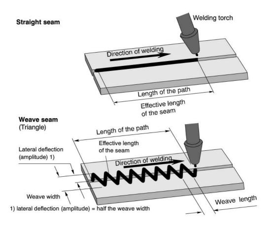
Trapezoidal, spiral and figure-of-eight weave patterns also result in a non-uniform effective weld velocity. This can vary between the set path velocity and a multiple of it during one period, depending on the relation of the lateral deflection (amplitude) to the weave length.
