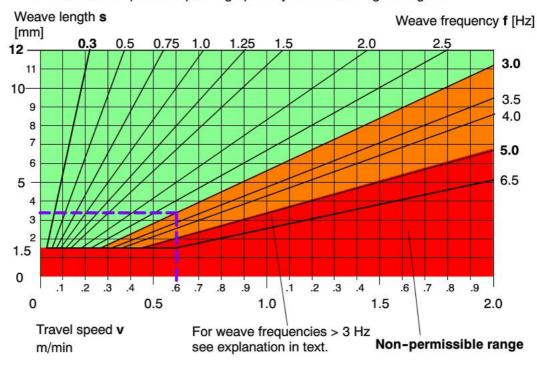
The maximum weave frequency for mechanical weaving is influenced by several factors, depending on the robot type concerned, for example by the resonant frequency of the "robot/tool" unit. Weave frequencies of up to 3 Hz (corresponding, for example, to a weave length of 3.33 mm at a travel speed of 0.6 m/min) are considered safe according to previous experience.
