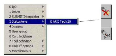
The configuration menu allows part of both the left status key bar and the softkey bar to be assigned specific arc welding functions by means of the menu item "Status keys". A graphic user interface optimized for the current application is thus available for the purpose of entering program commands and function calls.
