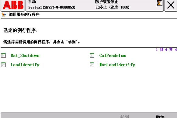
A screenshot of the 'Call Service Subroutine' dialog box. It lists four options: 'Bat_Shutdown', 'CalPendulum', 'LoadIdentify', and 'ManLoadIdentify'. The 'Bat_Shutdown' option is checked. At the bottom, there are '转到' (Jump) and '取消' (Cancel) buttons.                                                                                               |
